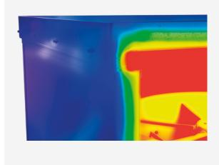
The new **HATCH/HP** has an extraordinarily low thermal transmittance coefficient:
