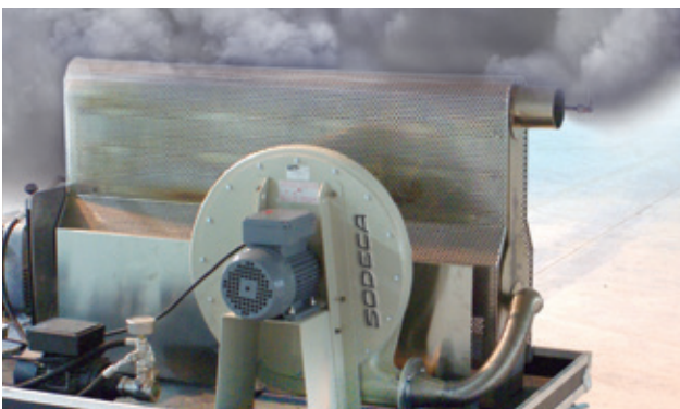
Smoke machine for conducting real smoke tests
